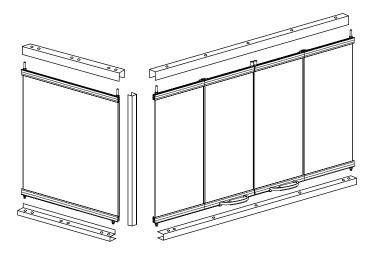
Lennox's Glass Door/End Panel Packaged Set, Models 38ACR and 38ACR-BB, are designed to be installed on the CR-3835R/L Series fireplaces. These kits come complete with all of the required hardware necessary to complete the task.
